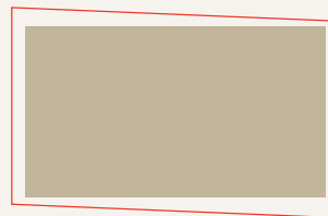
POOR BASE POSITIONING (CORNERS NOT AT RIGHT ANGLES)
